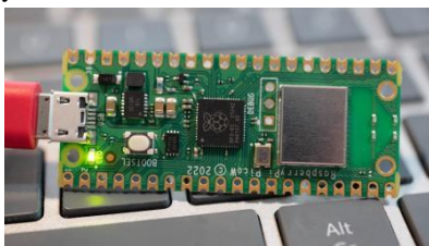
Figure 2: Raspberry Pi Pico W
